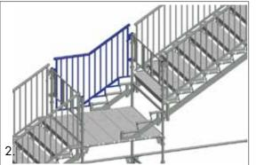
**2.** Insert handrail. Leave in the open and unlocked position.
