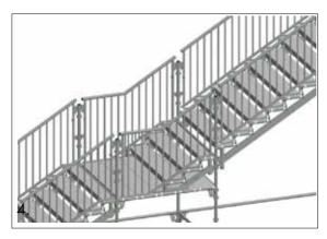
**4.** Once the stair is complete., remember to lock the handrail into place as shown previously.
