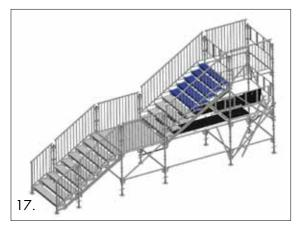
**17.** Standing on the decking units below fit the remaining treads in place.
