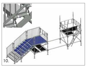
**10.** Secure the stair tread with the locking catch.
