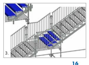
**3.** Slide the treads under the handrail and secure with the locking catch.
