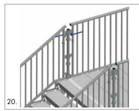
**20.** ! Once decking is complete all handrails **MUST** be dropped to their lowest position (locking all treads in place). Then all handrails must be fully secured by tightening the screw nuts at each end of the handrails.
