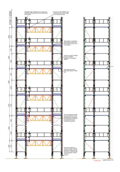
The Haki Tripod is designed for really demanding scaffolding jobs where leg loads are high. Permissible leg loads of up to 200kN can be achieved for propping and shoring applications.
